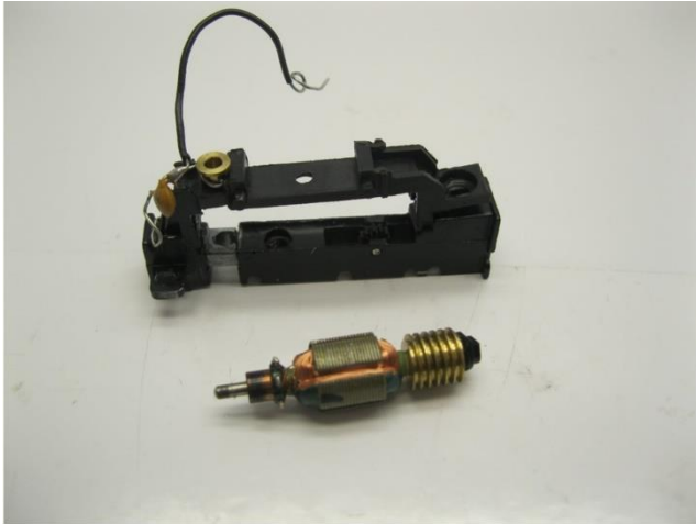
Ausbau alte Motor Take out the old motor Demonteer de oude motor
