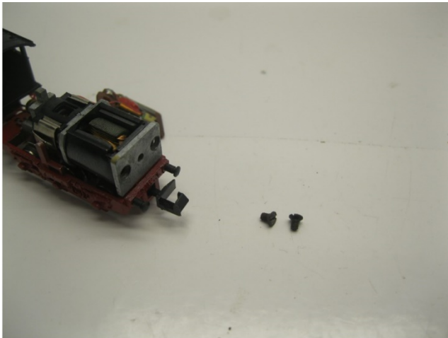
L Ausbau alter Motor Take out the old motor Demonteer de oude motor
