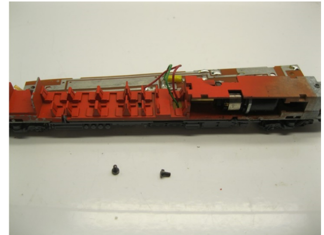
P Ausbau alter Motor Take out the old motor Demonteer de oude motor
