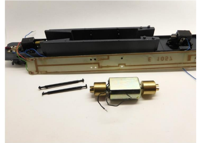
Ausbau alter Motor Take out the old motor Demonteer de oude motor
