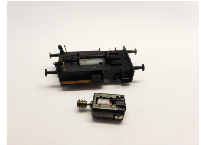
Ausbau alter Motor Take out the old motor Demonteer de oude motor
