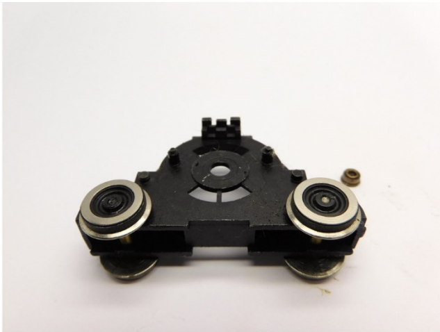
Ausbau Lager Take out bearing
