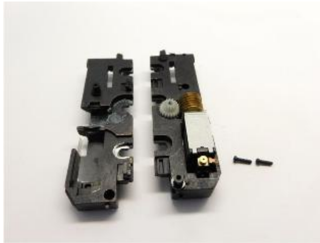
Ausbau alter Motor Take out the old motor Demonteer de oude motor
